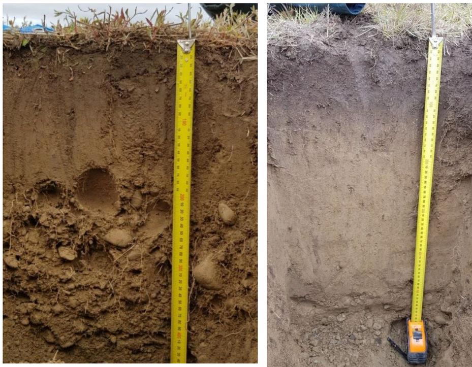
**Figure 4. Mackenzie Soil Phases. Left: shallow phase, depth to gravel 20 cm; Right: deep phase, depth to gravel 50 cm.**
